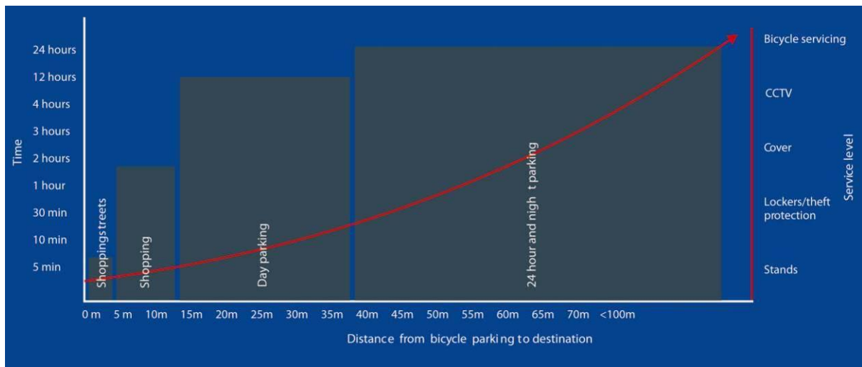
Acceptable distance from bicycle to various destinations (source: DCF, 2008 Bicycle Parking Manual, DK)
